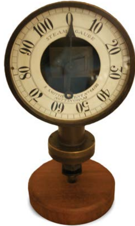
World's first Steam Pressure Gauge designed by Sydney Smith in 1847
