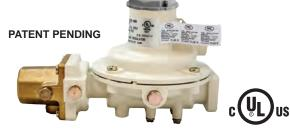
**MEGR-1232E Compact Series:** Offers a compact integral two-stage 2 PSI regulator design perfect for lower BTU applications and confined spaces. They feature an adjustment range from 1-2.2 PSI (factory set @ 2 PSI). Stainless steel integral components, fluorocarbon (FKM) seat discs, molded lip fabric reinforced diaphragms, and large precision machined aluminum orifices providing superior downstream regulation and maximum corrosion resistance against weather or contaminated gas.
