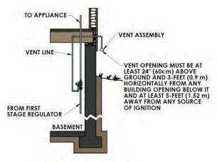
Figure 4: Basement Installation
