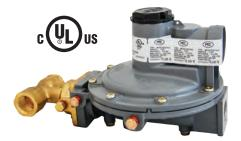
**MEGR-1632T Full Size Series**: Offers all of the same features as the compact MEGR-1232 series in a full size high capacity version. The full size MEGR-1632 diaphragm provides superior downstream regulation, has heavy duty wrench flats and a large 3/4" FNPT tapped drip lip vent to help prevent relief vent blockage.
