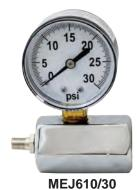
Designed to test low pressure lines for system leaks. The factory installed check valve allows the line to be pressurized and adjusted to the desired test pressure.
