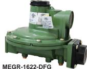
MEC full size second stage regulators have a large fabric reinforced diaphragm for superior downstream regulation, heavy duty wrench flats, and a large 3/4" FNPT tapped drip lip vent to help prevent relief valve blockage. The MEGR-1622 Series have both the inlet and outlet in line where the MEGR-1652 series have a rear discharge back mount outlet for convenient wall mount applications.
