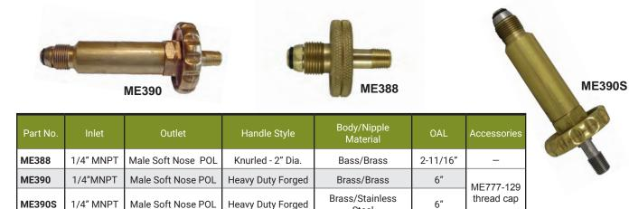
These adapters allow for quick conversion from a POL connection to various filling applications for retailers who fill multiple cylinder types through the same Type I (QCC) connection. Simply hand tighten the adapter to the POL filler connection (ME388 or ME390 Series).
