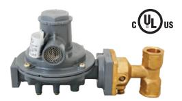
**MEGR-1232T Compact Series**: Offers a compact integral two-stage regulator design perfect for lower BTU applications and confined spaces. They feature an adjustment range from 9-13" WC (factory set @ 11" WC). Stainless steel integral components, fluorocarbon (FKM) seat discs, molded lip fabric reinforced diaphragms, and large precision machined aluminum orifices providing superior downstream regulation and maximum corrosion resistance against weather or contaminated gas.
