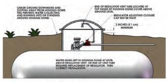
Figure 5: Underground Installation
