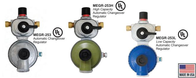
The **MEGR-253 Series** Automatic Changeover regulators automatically redirect LP gas vapor flow from an empty service cylinder to a reserve cylinder, without interruption of service. It features an easy to read green indicator which changes to red when the service cylinder needs to be refilled.
