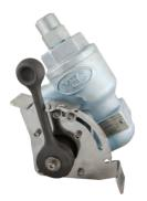
**Normal Bypass Mode**: functions just like our standard ME840 Series bypass valve during domestic tank deliveries by pushing maximum pump output to the hose end delivery nozzle while protecting the pump if the nozzle is closed during delivery. ERSAE ME845C-125 PATENT PENDING
